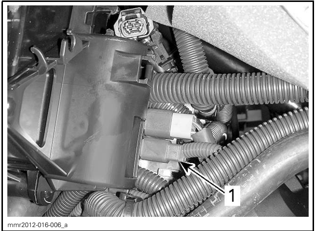
TYPICAL - RH SIDE VIEW 1. CPS sensor connector
