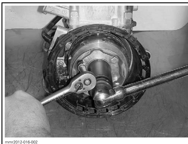
TYPICAL - STARTING PULLEY SCREWS REMOVAL
