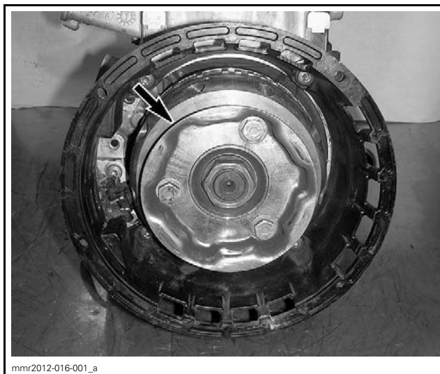
TYPICAL - STARTING PULLEY (800R E-TEC ILLUSTRATED)
