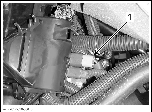
TYPICAL - RH SIDE VIEW 1. Stator connector
